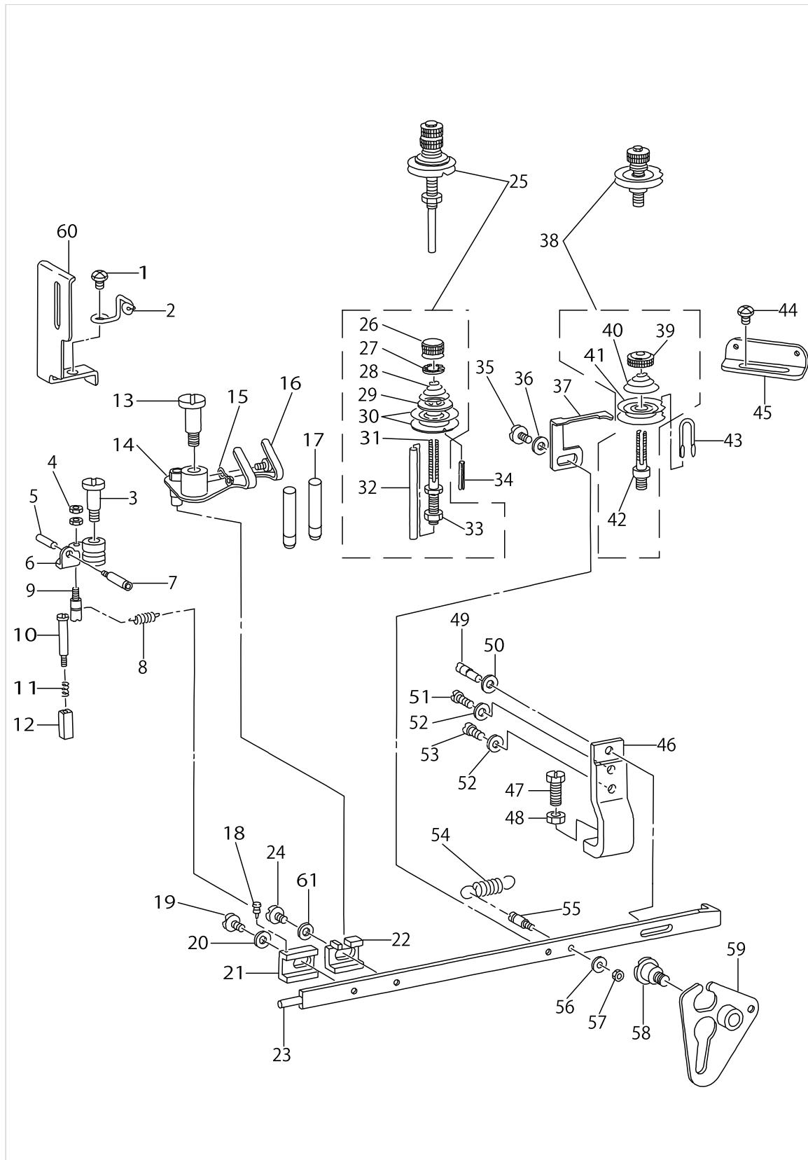
NIPPER & THREAD TENSION COMPONENTS
