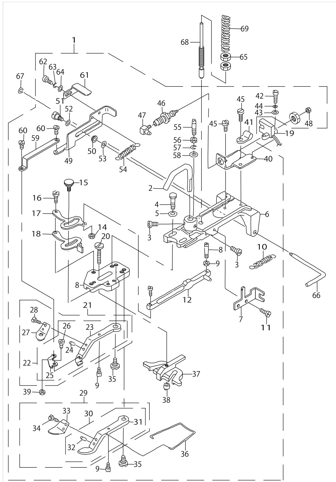
FEEDER CLAMP MACHANISM COMPONENTS
