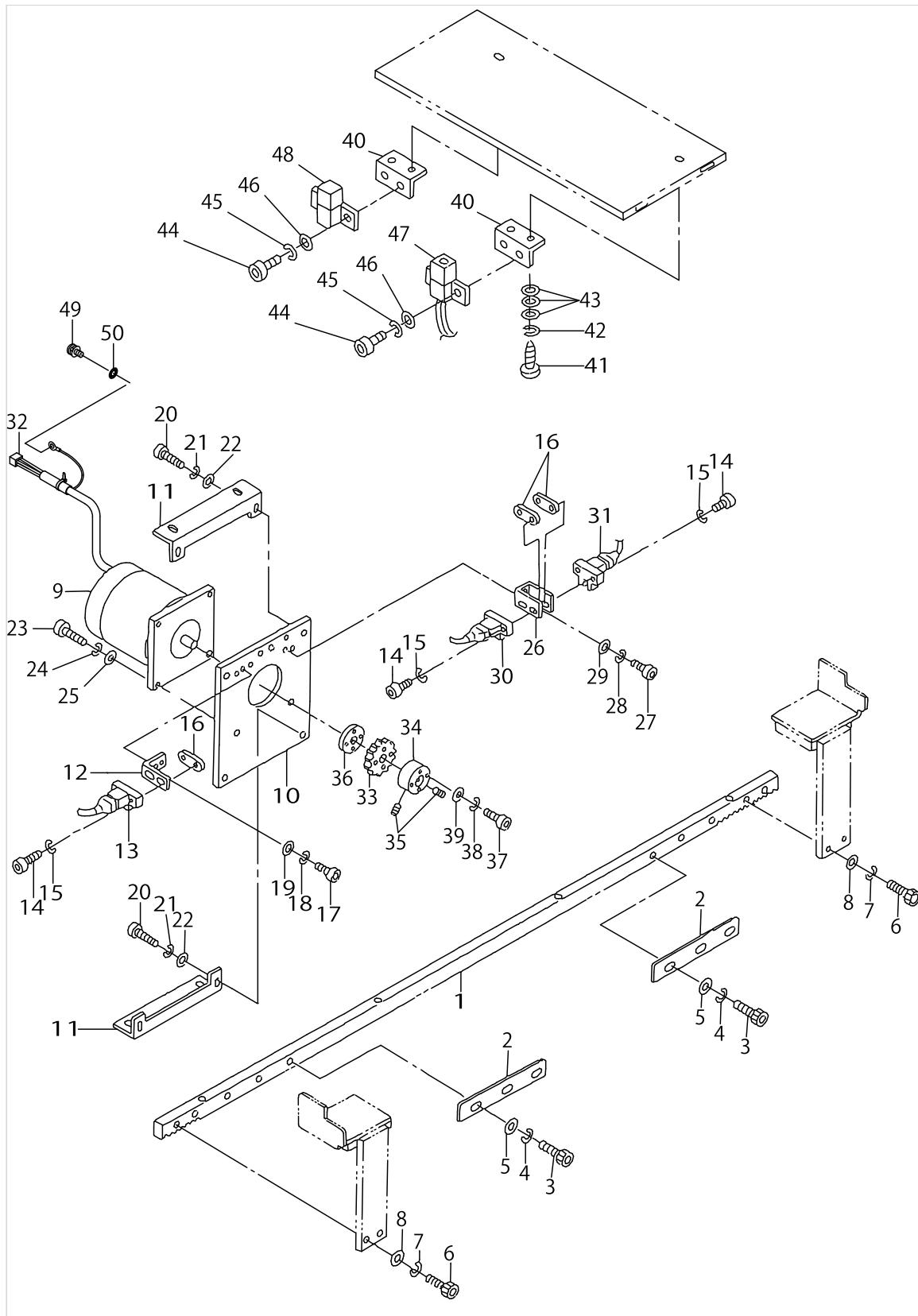
FEED MECHANISM DRIVE & SWITCH COMPONENTS
