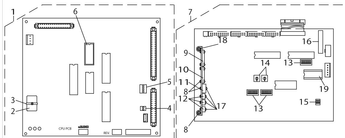
CPU CIRCUIT BOARD & I/O CIRCUIT BOARD COMPONENTS
