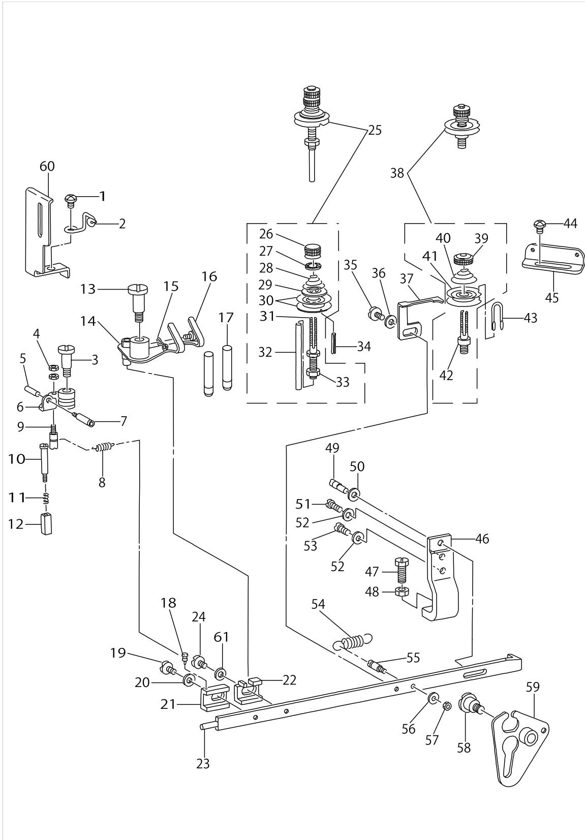
NIPPER & THREAD TENSION COMPONENTS
