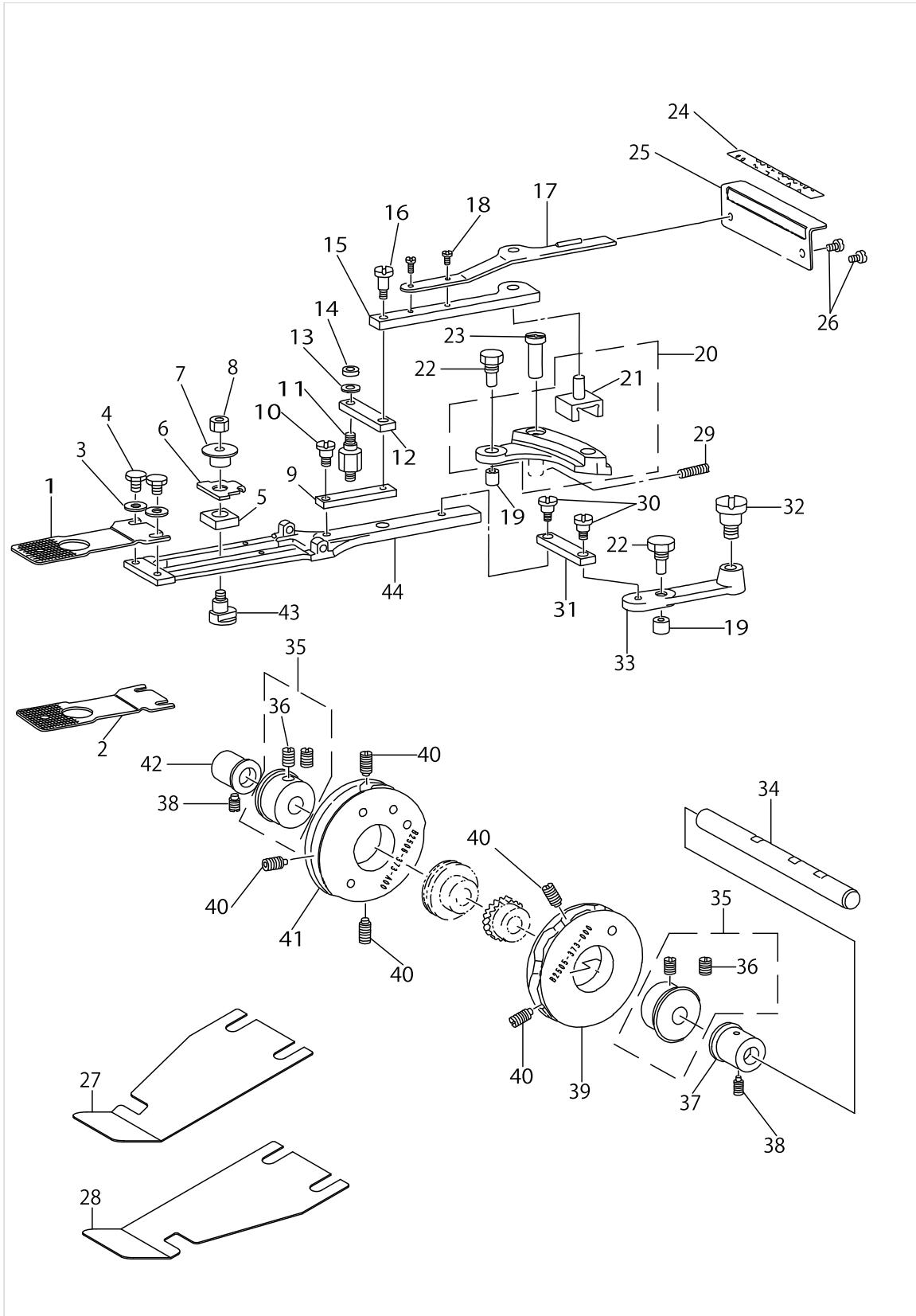
FEED MECHANISM COMPONENTS
